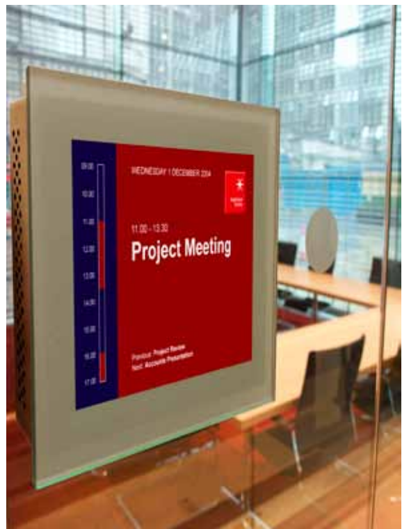
A standard RoomSign with a typical screen generated by Smart Sign Server integrated with a management database.
